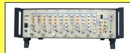
With applications such as AOC (Active Optical Cable) continuing to expand, this equipment offers multi-channel 10G BER testing at an affordable price.
