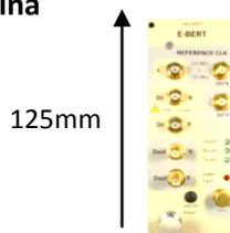
The new EBERT-5 is a Bit Error Rate Test module (PPG+ED) that plugs into the *XBERT* and *ParallelX™* Chassis. EBERT-5 can generate and receive electrical data from 8.0 Gb/s up to 11.3 Gb/s. Optionally it can also operate from 4.0 Gb/s up to 5.7 Gb/s (half-rate mode). EBERT-5 offers user programmable PRBS patterns, as well as variable output amplitude and crossover adjustment.
