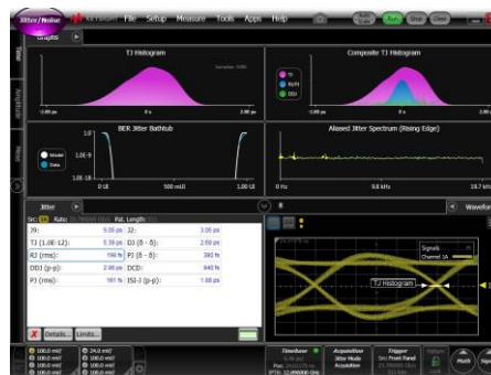
ELECTRICAL EYE-DIAGRAM PRBS9, Data Rate = 25 Gbps
